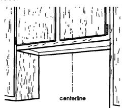
Determine and clearly mark a vertical centerline in the cabinet opening.
